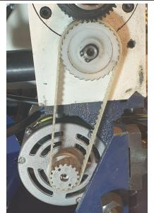
Fit the belt and adjust the tension using the bolts and nuts above the motor, ensuring that it is horizontal.
