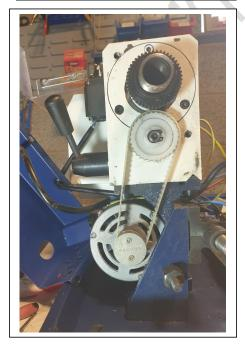
At this stage the process is complete, and reassembly can commence. However, I only replaced the motor cover and control unit, removed the chuck restraint before testing at low speed in Left and Right Hand drive.
