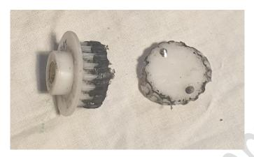
Removal of the end cover revealed that the plastic motor drive pulley had broken and the drive belt was not visible, but there was evidence on the pulley of it melting.
