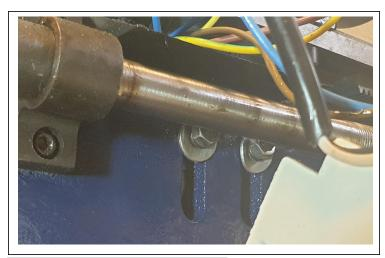
The motor retaining bolts are situated behind the leadscrew and can be slackened off using the 10mm open ended spanners.
