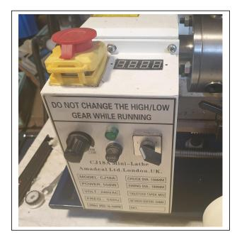
Undo the 4 posidrive screws, (2 at the top and two underneath. The unit can then be manoeuvred out of the way.
