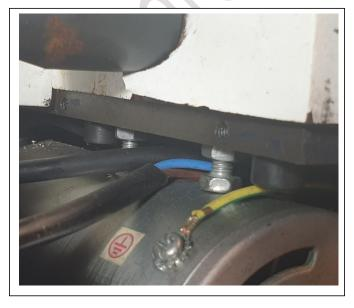
The 2 tensioning bolts are located above the motor. These can be adjusted using 2 x 10mm open ended spanners, preferably thin section. Undoing the top nuts allows the bolt to be screwed into the bottom of the headstock casting. Slacken both off.
