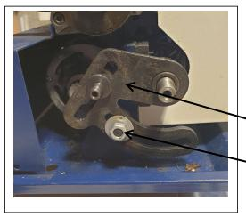
Remove the M14 nut and washer and the bottom gear support bracket.
