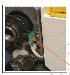
Remove the small PCB holding the Hall Effect Transducer (RPM pickup). Slacken off the round head screw and it slots off.
